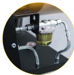
Fuel preheater is optional, fuel filter is outside
